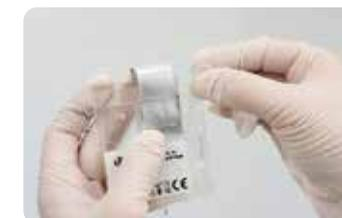
2. Insert the capillary holder into the cartridge
