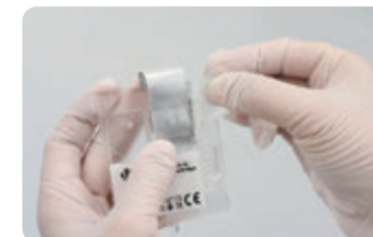
2. Insert the capillary holder into the cartridge
