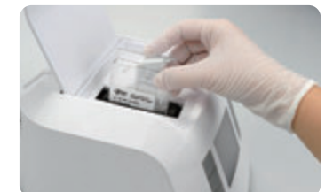
3. Insert the cartridge, pull the tab and close the lid
